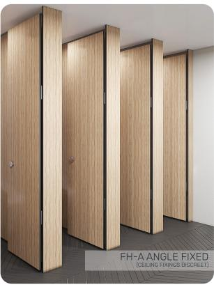
The FH Full Height partition system is the perfect system for complete cubicle privacy. The FH system has floor to ceiling panels and doors with clearances of 20mm FFL and 80mm FCL. The 80mm clearance at the top of the doors allows the lift off hinges to function in case of emergency. The FH partition system is the next best thing to an individual room but at a fraction of the cost.
